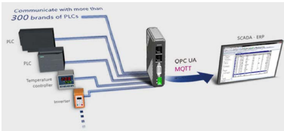
Figure 1. The integration of numerous proprietary plant-floor protocols remains an important function at the interface between OT and IT systems
