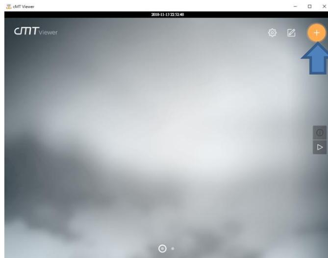
Search for cMT HMIs on [Search] tab. The available HMIs will be shown as below when existing on the local network. Tap an Add icon on the desired HMI, and it will bring up a window requiring you to enter the password.
