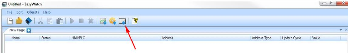
3. Click on the Add button to add an existing cMT HMI. Enter its IP address and port number.
