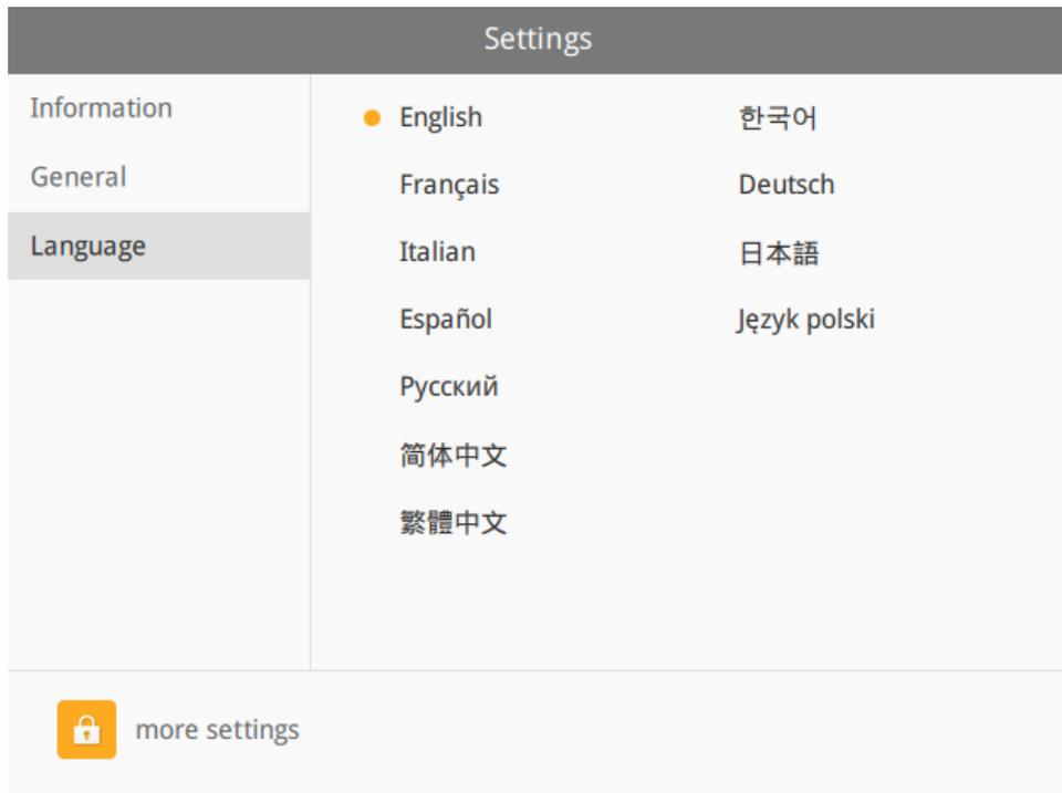
To enable Monitor Mode and use Password Protection functionalities, click on “more settings” icon and log in with the password set on “Change password.” The default password is 111111. There are more options available on the **General** tab and the **Password Protection** tab.
